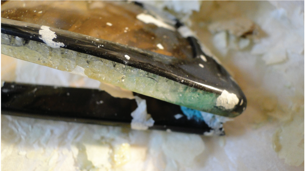
Figure 2.1 A cellulose nitrate spectacle frame showing the sugar effect. From the collection of Kunstmuseum Den Haag. © Carien van Aubel.
