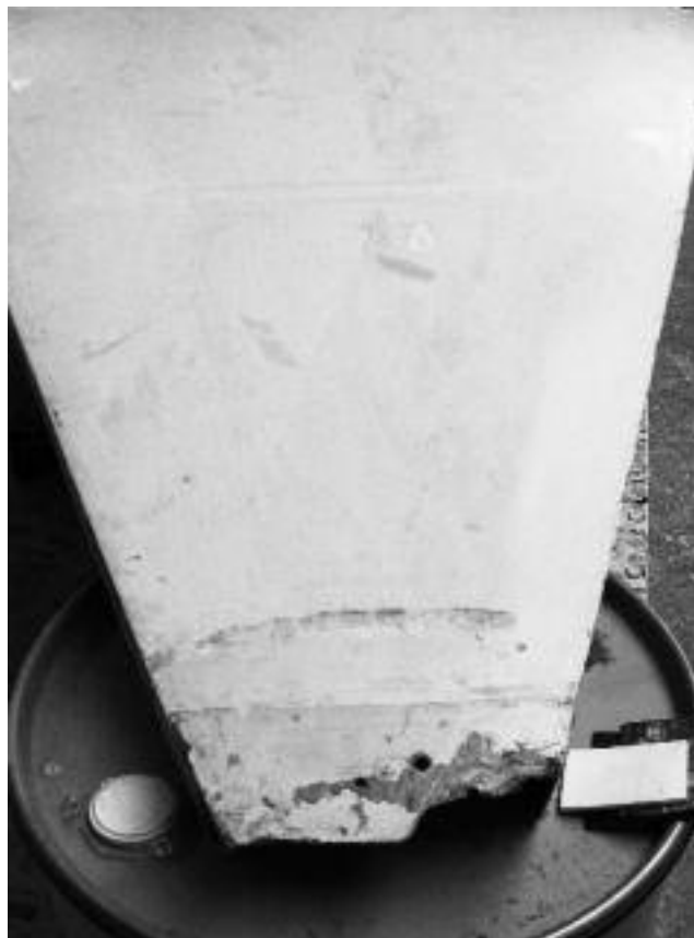
Figure 4 Detail of one of the shell elements; halfway the surface cleaning treatment
