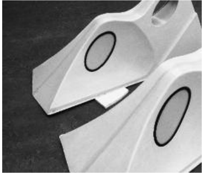
Figure 8 Two fiberglass reinforced polyester elements from the seats in the living room
